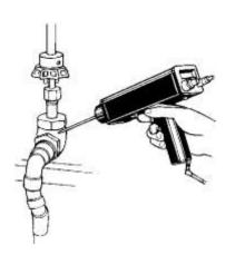
CHECKINGVALVE LEAKAGE/ BLOCKAGE WITH THE ULTRAPROBE
