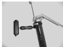
2. Connect cable from Sensor Assembly to input of Grease Caddy.
