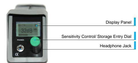
**SENSITIVITY/STORAGE ENTRY CONTROL DIAL.** This is the most important control in the unit. It is used to adjust the sensitivity. When clicked, it changes functions such as store data or change the storage location number. It is also used to get into the "SET UP" mode (described later).
