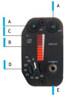
(C.) **Battery Level Light.** This red light turns on only when the batteries need to be recharged.
