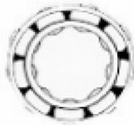
Lack of Lubrication Increases amplitude levels
