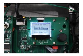
**<u>29. System Shutdown Continued.</u>** To keep the system on-line, Click/push to enter, select "**No**" and push the dial to exit shutdown mode.
