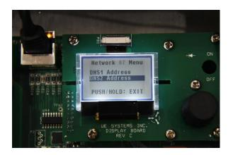
**<u>26. DNS2 Address Cont.</u>** Spin dial to desired number, push dial to activate and spin again to modify. Once modified, push dial and spin again to "exit" and push to exit out of screen.
