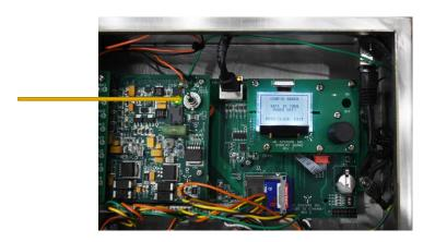
**32.** Display 2: Make sure that "Display 2" is being displayed and push and hold the sensitivity knob.
