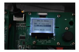
**<u>12. DMS IP Port:</u>** Is the port number that the UE Server is configured to and connects with on the database computer. Spin the dial to the correct # you want to change and then push the dial. Next, spin to the desired value. When finished, highlight EXIT and hold down the dial to exit out of the menu.
