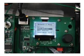
**<u>24. DNS1 Address Cont.</u>** Spin dial to desired number, push dial to activate and spin again to modify. Once modified, push dial and spin again to exit and push to exit out of screen.
