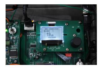
**<u>28. System Shutdown</u>**: Push the Sensitivity knob to activate the menu.
