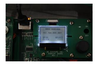
**<u>27. DMS Connected</u>**: Once configuration for the network is complete and correct (for both the UE Server and UE 4Cast), the top of display will state that DMS is now connected to the 4Cast box.
