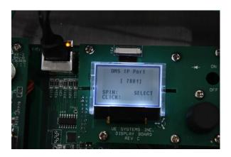
**<u>13. Network Menu:</u>** Inside this menu is where to configure the network of 4Cast. Push/click the knob to enter.
