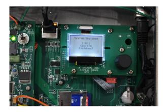
**<u>30.System Shutdown Continued</u>**: To turn the 4Cast system off, select "**Yes**" and push the dial to confirm shutdown.
