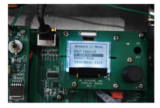
**<u>18. IP Address Cont.</u>** Spin dial to desired number, push dial to activate and spin again to modify. Once modified, push dial and spin to exit and push to exit out of screen.
