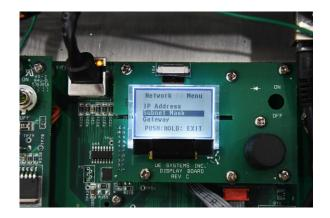
**<u>20.Subnet Mask Cont.</u>** Spin dial to desired number, push dial to activate and spin again to modify. Once modified, push dial and spin again to "exit" and push to exit out of screen.
