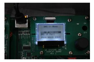
4.) <u>Modify Address</u>: Spin the dial to the desired number, push/click the dial select and then spin again to modify. Once modified, push and spin again to exit and push again to exit out of screen. Again, the IP Address on the 4Cast needs to match the IP Address of the of the UE Server computer so that both "UE server" & 4Cast can communicate.
