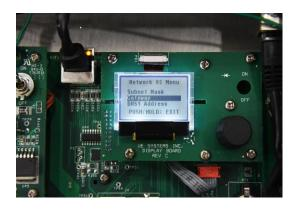
**<u>22. Gateway Cont.</u>** Spin dial to desired number, push dial to activate and spin again to modify. Once modified, push dial and spin again to "exit" and push to exit out of screen. Typing ipconfig within the CMD prompt on the computer that will run the UE Server will give you the correct "Gateway" address.
