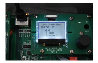
**<u>33. Display 2 Continued</u>**: Once Display 2 is enabled, the screen will display all 4 sensors with current "live" decibels and sensitivity levels.
