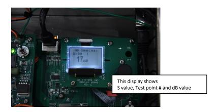
4. <u>Setup Menu</u>: Push (click) the sensitivity knob until the bottom of screen is flashing and spin the sensitivity knob until "Setup Menu" is present. Push and hold the sensitivity knob in place until you are in the setup menu options.
