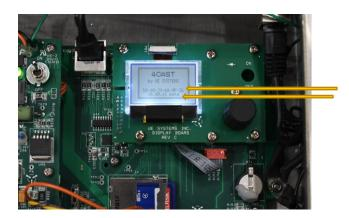
3. Once the boot sequence is finished, it will show the "main" display: The sensitivity value "S=", Point # and dB of the sensor. If 4Cast is not reading correctly, the display will show an arrow pointing to the left, meaning over-range or an arrow pointing to the right meaning under-range.
