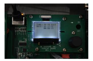
**<u>8.</u>** <u>Menu #2- DMS Menu:</u> The section holds the IP Address and IP Port information. Highlight DMS Menu and hold down the dial to enter.
